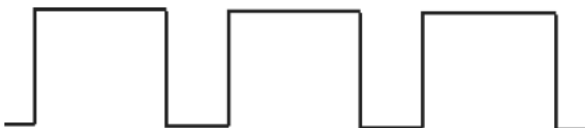
Forward power sensor signal waveforms
